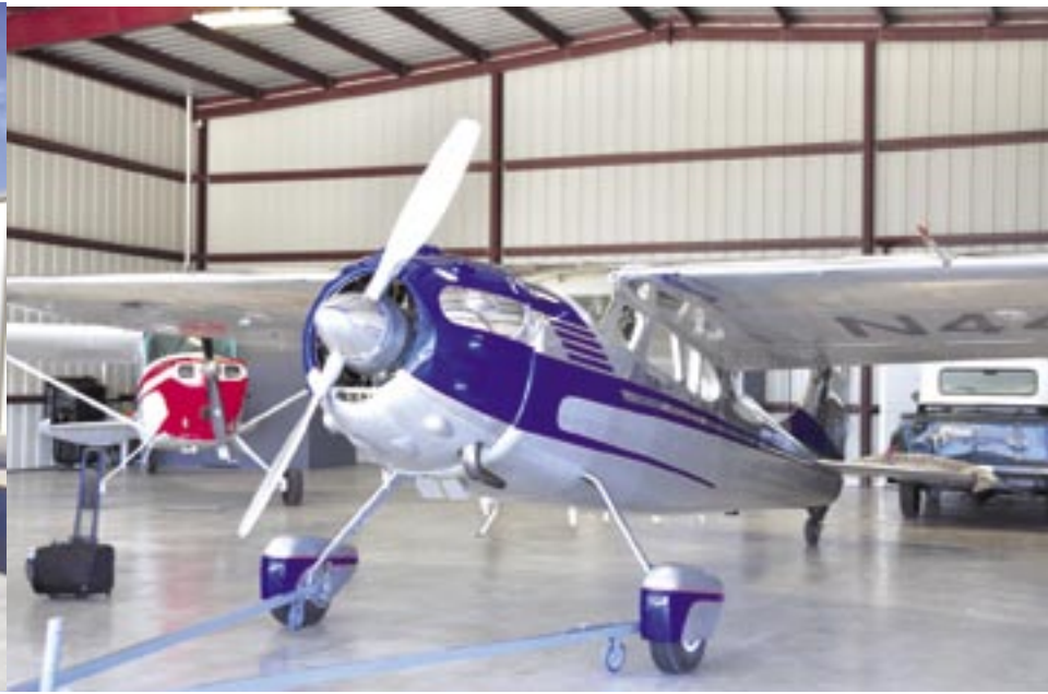
The 195 Businessliner is Cessna's only postwar aircraft with a radial engine. Photo: John Weisbart.
